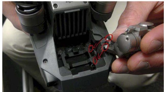
ILLUSTRATION 1.—Gimbal Mounting Plate Breaking Point
